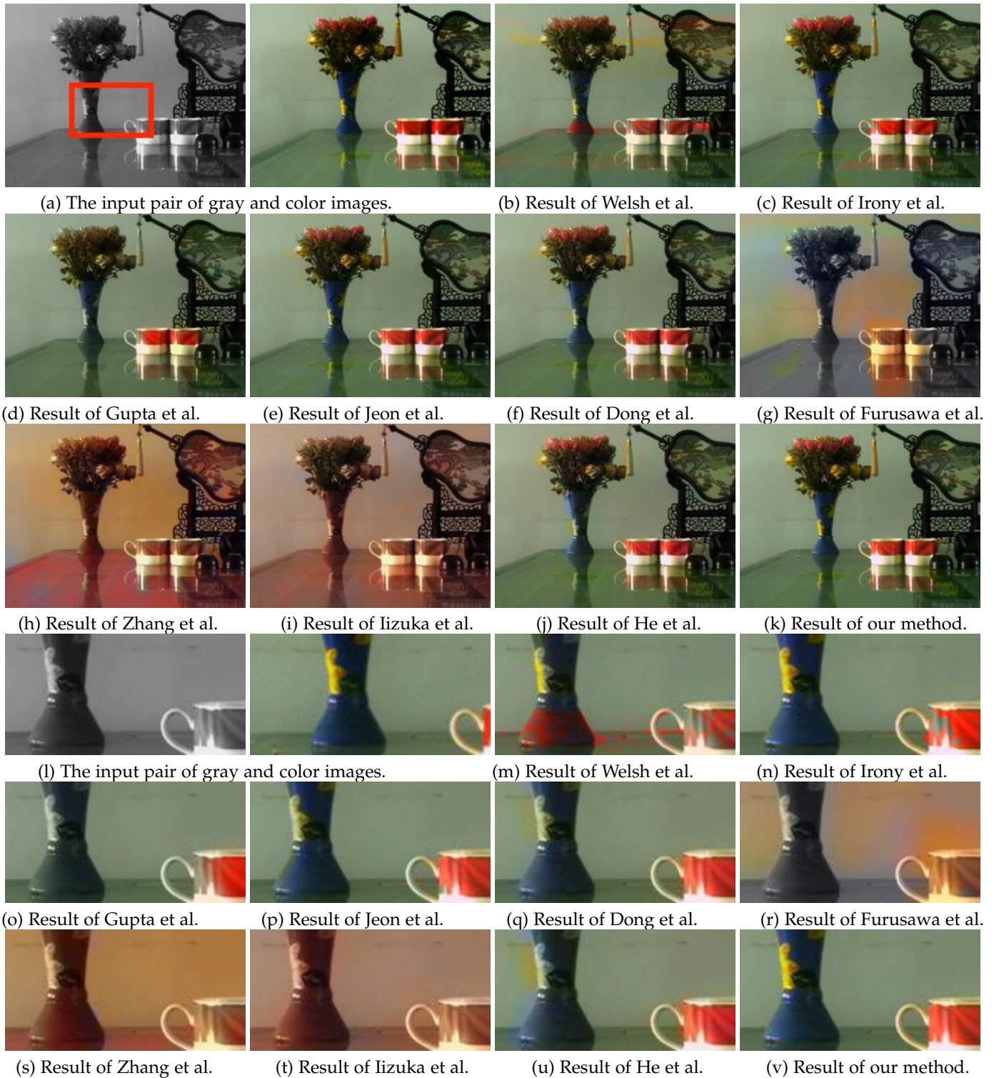
Fig. 13. Examples to compare the colorization results of all the comparison methods and our colorization method. The region marked with the red box is enlarged in the bottom three rows. The input images are captured by the real monochrome-color dual-lens system of Huawei P9 phone.
