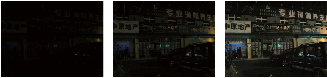
Fig. 5 Example of enhancement with and without adaptive exposure adjustment. a) Input image; b) Middle: recovered image without adaptive exposure adjustment; c) Recovered image with adaptive exposure adjustment
