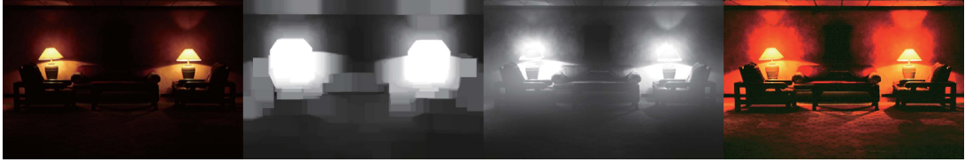
Fig. 4 Example of transmission value correction. (a) Input low lighting image; (b) estimated transmission map; (c) refined transmission map after transmission value correction; Final low lighting enhancement image
